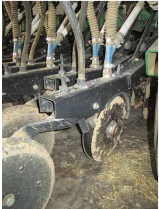
Figure 4. On the disc opener of this grain drill, the tube from the small seed box (smooth tube) deposits seed behind the disc opener for shallow seed placement. The tube from the large seed box (corrugated tube) deposits seed at the front of the disc opener for placement at the bottom of the furrow.
